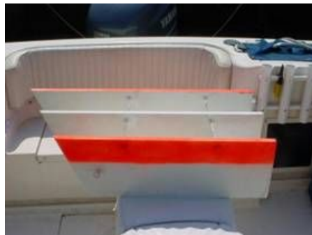
Figure 36. The three-board planar board design selected for initial prototyping, testing, and evaluation.
